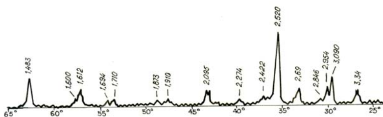
Fig. 2. X-Ray of the used magnetite (Fe 3 O 4 ) micropowder
