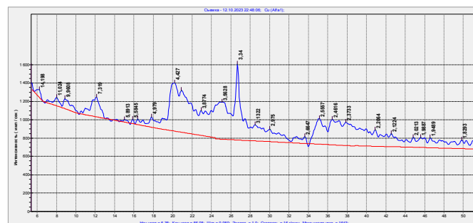
Fig . 5. Village Mamati Clay Sample X-ray
