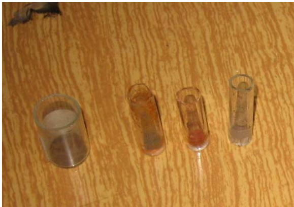
Fig. 11. Test tubes made of glass pipe
