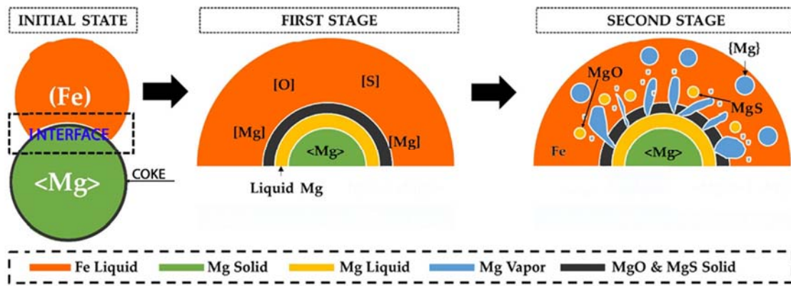
Figure 1. Schematic model of modification by permeable porous composites of liquid metal with Mg vapors
