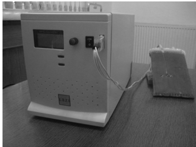
Fig. 1. Clinical medical device for the treatment of tumors of internal organs, skin and subcutaneous tissue "LEZI 1" for controlled local hyperthermia, created at the Bionanoceramic and Nanocomposite Materials Science Center of Georgian Technical University (manager: Prof. Z. Kovziridze)
