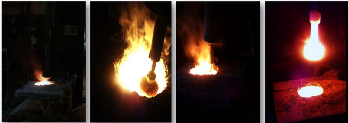
Figure 2. Technological process of modification of Mg cast iron
