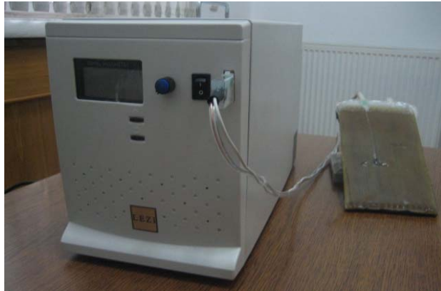
Clinical therapeutic device “Lezi 1” created at the Bionanoceramic and Nanocomposite Materials Science Center (manager Prof. Z. Kovziridze) of Georgian Technical University for Treatment of skin and subcutaneous cancer diseases by controlled local Cancerthermia.
