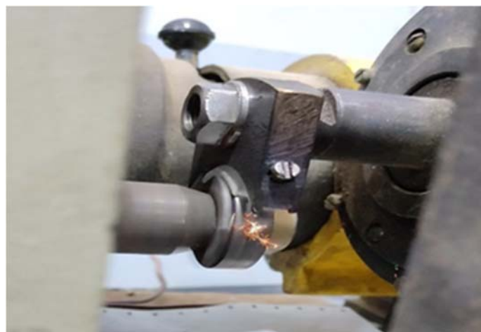
Fig. 2. Testing samples on a tribometer
